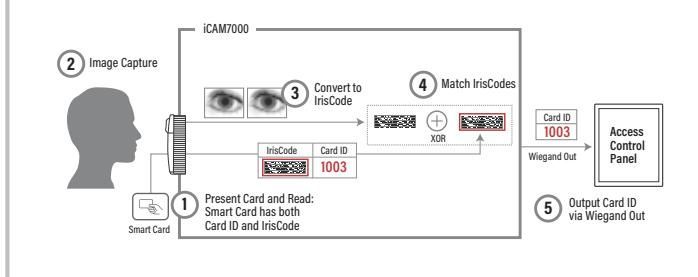
The verified card ID is output to the 3rd party access control system. This operation does not require a network connection.
