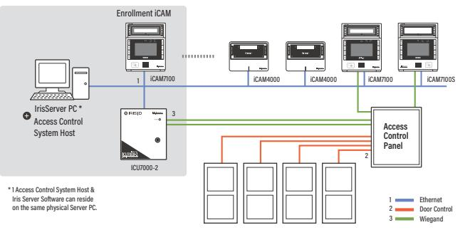
DES and 3 DES encryption options are available. The 3 DES encryption can be set by the end user. Note: The ICU7000-2 is offered as an optional solution for off device matching.
