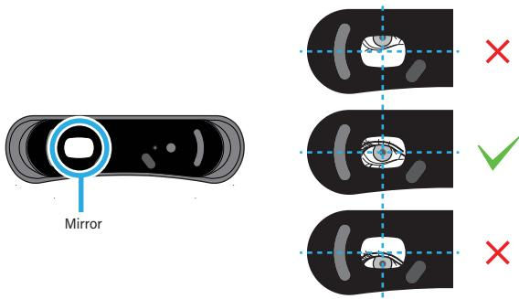
**NOTE** If looking into the mirror with the left eye is not possible or uncomfortable; the user may position the right eye straight at the right eye indicator LED. The unit operator may assist in directing you during this process.
