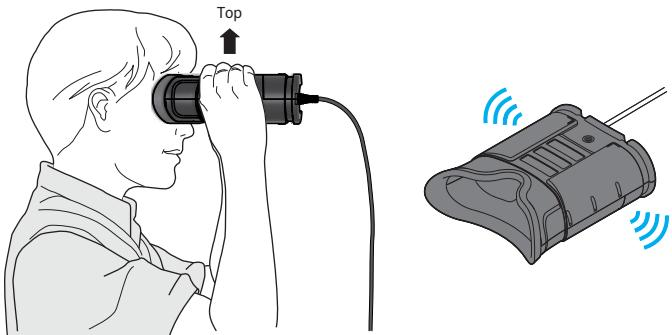
**NOTE** This product contains a built-in orientation sensor to assure proper usage. If the T10 is in an upside down position for usage, the unit will beep repeatedly until the correct orientation is restored.
